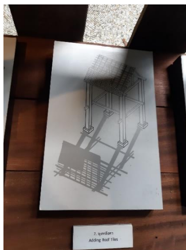
Remembering craftsmanship and methods in vernacular wood construction: Inside the Lanna Traditional House Museum (Chiang Mai University), one of the illustrations depicting various stages and elements of house construction (Photo: Christine Richter, Fraunhofer IMW)
